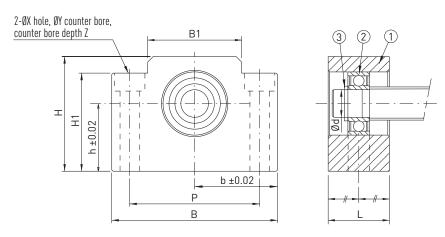
(1) Housing, (2) Bearing, (3) Circlip
