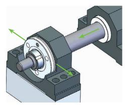
Fig. 4.10 Fixed bearing with applied constraining forces
