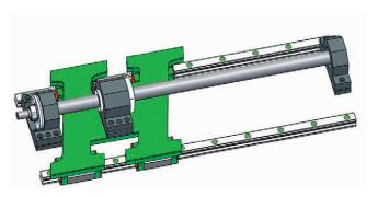
Fig. 4.9 Ballscrew at the left stop for aligning the fixed bearing
