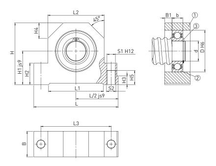
(1) Steel pillow block housing, (2) Bearing, (3) Circlip
