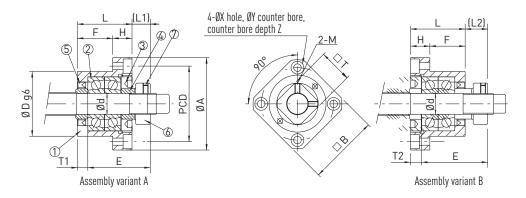
(1) Housing, (2) Bearing, (3) Retaining cover, (4) Support ring, (5) Seal, (6) Clamping nut, (7) Allen set screw
