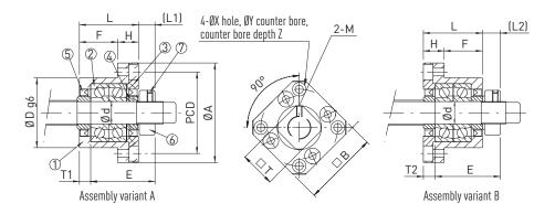
(1) Housing, (2) Bearing, (3) Retaining cover, (4) Support ring, (5) Seal, (6) Clamping nut, (7) Allen set screw
