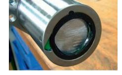
Fig. 4.6 Screw nut with wiper onto shaft
