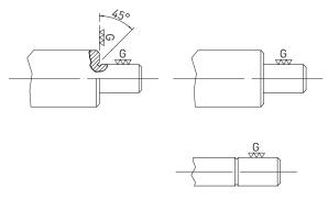
Fig. 7.3 Recesses for avoiding peaks in stress
