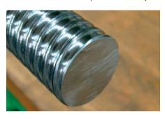
Fig. 4.3 End of shaft before the NBR wiper is assembled
