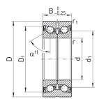
Acting on two sides Series ZKLN...2RS, ZKLN...2Z
