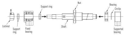
Fig. 4.8 Exploded view of the ballscrew with bearing units
