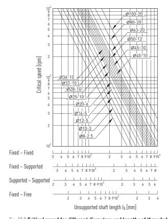
$\label{eq:Fig. 10.3} \textbf{Critical speed for different diameters and lengths of threaded shafts}$
