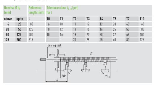
Table 4.3 Radial runout  $t_{6.2}$  of bearing seat related to the centre line of the screw part (measurement in accordance with DIN ISO 3408)
