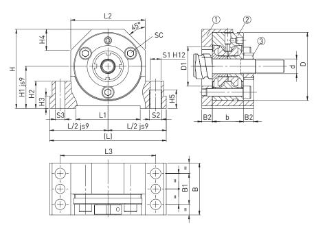
(1) Steel pillow block housing, (2) Bearing, (3) Lock nut
