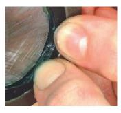
Fig. 4.7 Fixing the wiper while slowly screwing nut onto shaft
