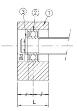
(1) Housing, (2) Bearing, (3) Circlip
