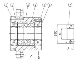
(1) Mounting bolt, (2) Bearing cover, (3) Bearing housing, (4) Bearing, (5) Seal, (6) Spacer, (7) Lock nut
