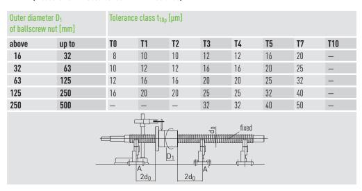
Table 4.10 Parallelism deviation t<sub>11</sub> of rectangular ballscrew nut related to AA' (for preloaded ballscrew nuts only) (measurement in accordance with ISO 3408)
