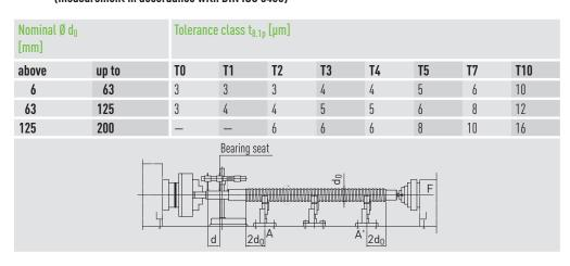
Table 4.7 Axial runout t<sub>8.2</sub> of the shaft faces related to the centre line of the screw shaft (measurement in accordance with DIN ISO 3408)
