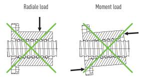
Fig. 4.1 When installing the ballscrew, there must not be any radial or eccentric forces acting on the nuts or shafts
